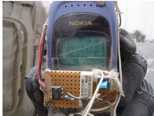
Figure 6: An image of a cell phone triggered IED that did not successfully detonate. (Image Source: Jacob Appelbaum)
